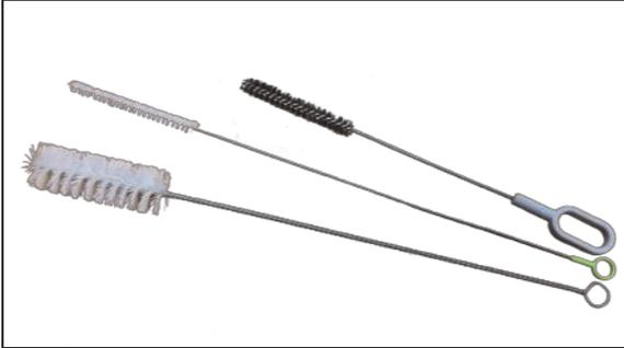
**Twisted-in-wire Brushes** are commonly referred to by our customers as twisted brushes, tube brushes, bottle brushes or pipe brushes. Twisted-in-wire brushes are made by placing filament material in between the stem wires and then twisting the stem wires tightly to secure the filament.
